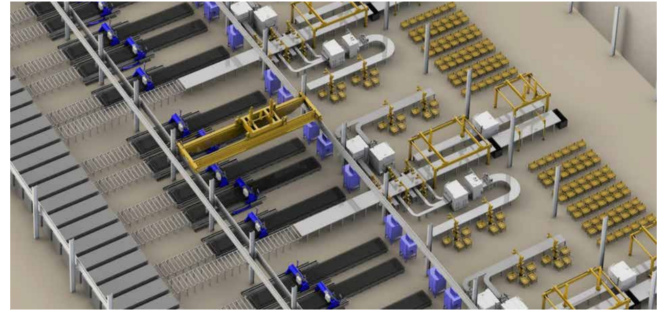
Automatic plasma cutting & sorting line with heavy-duty storage tower
